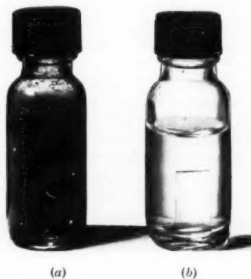
Fig. 1 Uninhibited and inhibited steel corrosion. The specimens contain 10 ppm of chloride ion. (a) Corrosion in distilled water. (b) Inhibition of corrosion by pertechnetate ions.
